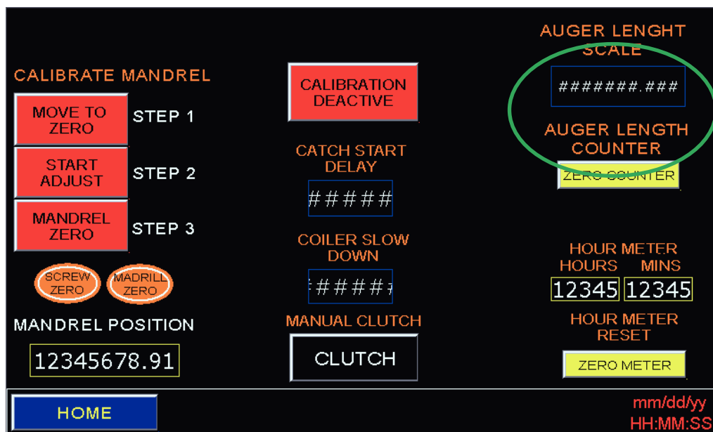
Figure 15: Calibration screen on HMI
